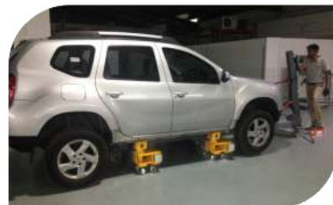
Vehicle is now clamped to MINI 10 and ready to repair using the hydraulic pulling tower operated by a Pneumatic foot pump.
