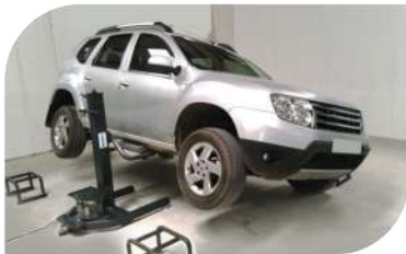
Jack up the vehicle using the lift (or use a trolley jack) and place on the wheel stand.
