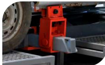
Slide the sill clamp
