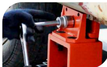
Fasten the sill clamp and raise the bench
